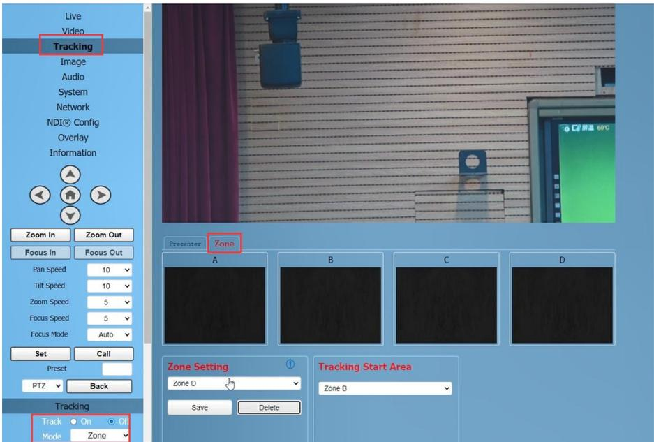
**Step 3** Use the web interface's directional keys and Zoom In/Out to adjust the lens position,
