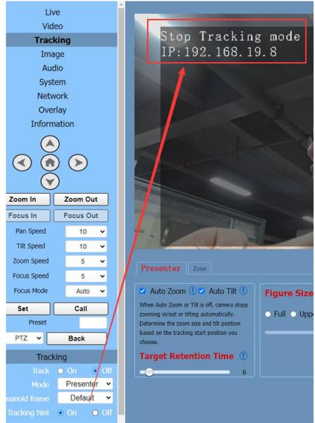
**Step 6** Turn on tracking, press the arrow keys to select the tracking target, and then press Home to confirm.
